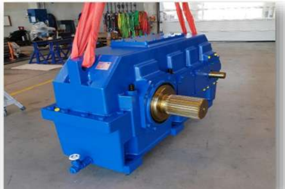
Assembly of the new manufactured gear set with new bearings, after measurement and re-engineering of the old gear set.
